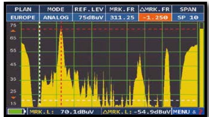
C/N measurement mode "OUTSIDE THE BAND": The signal/noise ratio is measured between the signal level of the video carrier (signal/carrier, red marker) and the noise level estimated in the guard band (-1.250 MHz from the video carrier, white marker)
