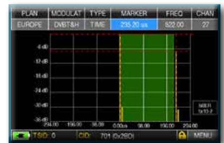
Fig. 3: MARGINAL RECEPTION (or IMPOSSIBLE):* 2 ECHOES present outside the guard interval mask (green area), coming from a distance of: 1st echo: 70,56 Km, the same as a 235,20 \mu\text{s} delay.
