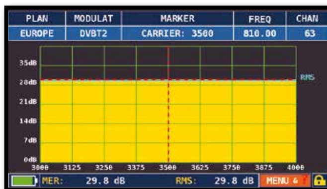
MER vs CARRIER: Visualization mode "VIS. TYPE: NORMAL", "PICTURE: FULL" and "START/STOP CARR from 3000 to 4000".
