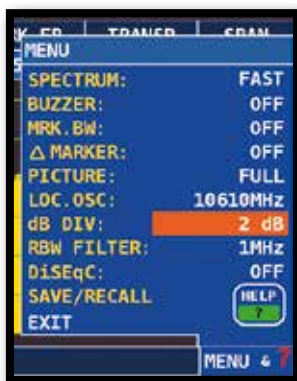
Touch "MENU&?" from the SAT SPECTRUM screen, select "dB DIV 2dB" and "RBW FILTER 1 MHz".
