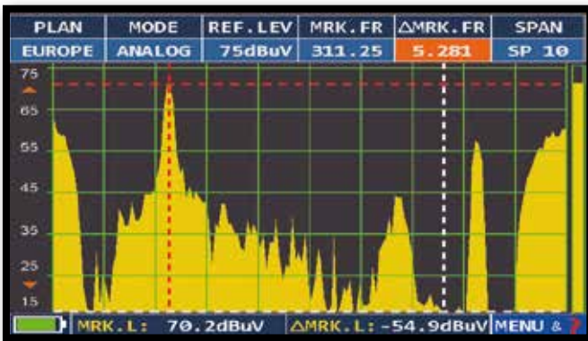
C/N measurement mode "IN BAND": The signal/noise ratio is measured between the signal level of the video carrier (signal/carrier, red marker) and the noise level, estimated in the band between the coloured subcarrier and the audio carrier (white marker)
