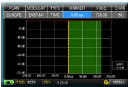
Fig. 1: OPTIMUM RECEPTION:* no ECHO present either outside or inside the guard interval mask (green area).
